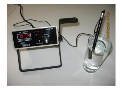
In this picture, we are measuring the ionic strengths with our Amber electrical conductivity meter. It reads 1.4 Micro-Siemens which is a little high but still pure enough for making colloidal silver. Please note that the reading will vary depending on the quality of your distilled water.
