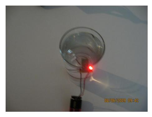
It is now a bit more than two hours later and we can see that the LED is glowing much brighter, indicating that we are running a much higher current than when we started. This indicates that we have generated enough ions to increase the conductivity of the water.
