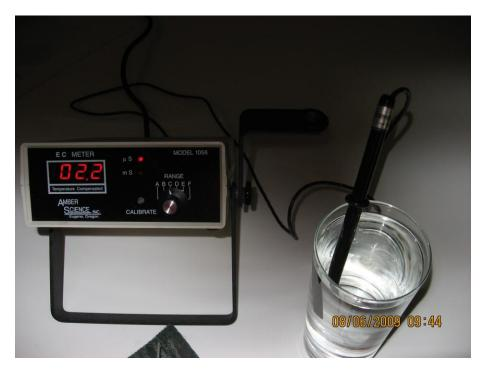
This is confirmed by measuring the PPM of the water in the glass. It reads slightly over two PPM. So we continue the process.
