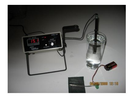
We confirm this with the use of our electrical conductivity meter. It reads 15.1 PPM. Please note that the reading will vary depending on the quality of your distilled water. We are now finished with the process of making our colloidal silver.
