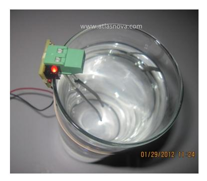
This picture shows that the LED is less bright after we moved the position of the silver wires, so we let the process continue.
