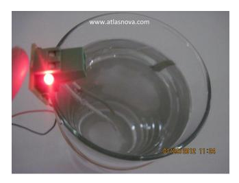
Around two hours later, we can see that the LED is glowing brighter, indicating that we are running a higher current than when we started. This indicates that we have generated enough ions to increase the conductivity of the water.
