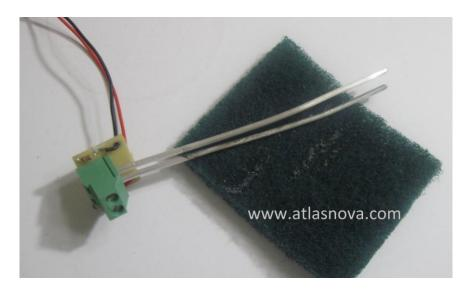
We are now finished with the process in making colloidal silver. Unplug the universal power supply, remove the generator from the water and clean the silver wires with a scrubbing pad. Two or three swipes should suffice.
