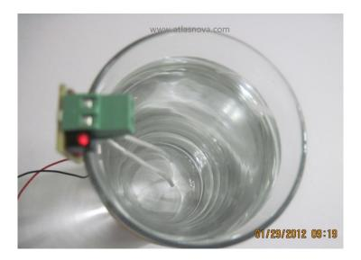
Place the generator on the rim of the glass as shown in the picture. Make sure that the silver wires are not touching each other. Position the printed circuit board (generator) on the rim of the glass in such a way that the ends of the silver wires in the water are near the center of the water, and keep the silver wires at least 1 inch away from any glass surface in the water. Also, make sure that any part of the generator (printed circuit board) is not touching the water.
