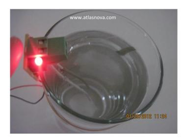
Around two hours later, we can see that the LED is glowing brighter, indicating that we are running a higher current than when we started. This indicates that we have generated enough ions to increase the conductivity of the water.
