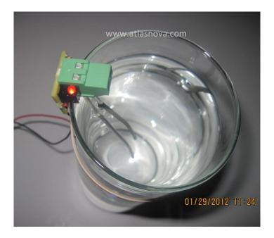
This picture shows that the LED is less bright after we have moved the position of the silver wires, so we let the process continue.
