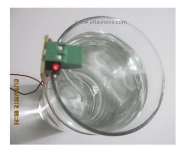
We can see that the LED is only faintly glowing. If it glows any brighter than this, it would indicate that the water we are using is not of the purity required for making colloidal silver.
