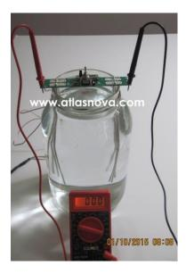
Put the two test leads into the two outer test points on the generator as shown. The meter should read zero volts.
