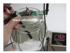
In this picture we have submerged the probe of our Amber Electronic Conductivity Meter to measure the value of conductivity in Microsiemens. (Please note that our toggle switch is in UPRIGHT position). This is the same value for the PPM (parts per million) of the ionic part of our colloidal silver. As you can see in our picture, our PPM reads 16.2.
