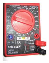
Plug the test leads into the Multimeter at the two lower sockets on the meter. The top socket is not used. It is only there for measuring very high amperage.
