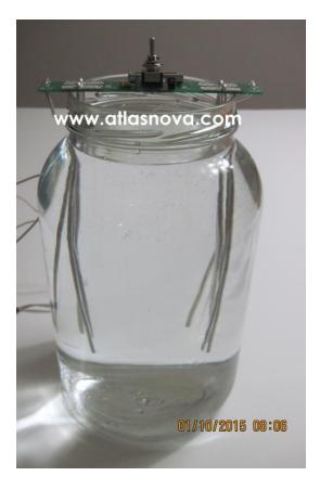
Place the printed circuit board (generator) with the silver wires on to the jar. Make sure that none of the silver wires are touching any part of the jar where the water is present. The silver wires should be as far apart as possible.
