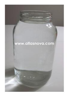
Then dispose off the water. Pour distilled water into the jar. Do not fill the jar beyond 1 inch below the top of the jar.
