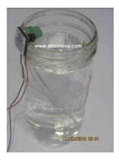
Slide the rubber band onto the jar to make sure that the silver wires are not touching the jar itself. This is to hold the silver wires in the center of the solution.
