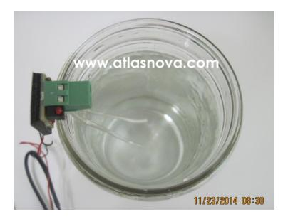
Place the generator on the rim of the jar as shown in the picture. Make sure that the silver wires are not touching each other. Position the printed circuit board (generator) on the rim of the jar in such a way that the ends of the silver wires in the water are near het center of the water, and keep the silver wires at least 1 inch away from any glass surface in the water. Also, make sure that any part of the generator (printed circuit board) is not touching the water.
