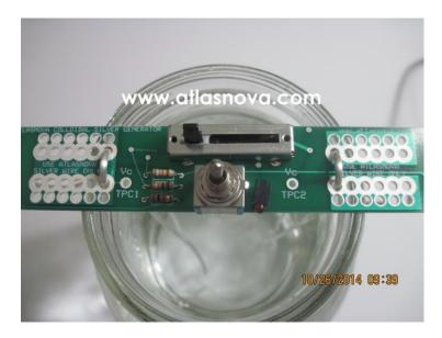
Place the printed circuit board (generator) with the silver wires on to the jar. Make sure that none of the silver wires are touching any part of the jar where water is present. The silver wires should be as far apart as possible.
