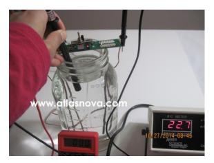
In this picture we have submerged the probe of our Amber Electronic Conductivity Meter to measure the value of conductivity in Microsiemens. (Please note that our toggle switch is in UPRIGHT position). This is the same value for the PPM (parts per million) of the ionic part of our colloidal silver. As you can see in our picture, our PPM reads 22.7.
